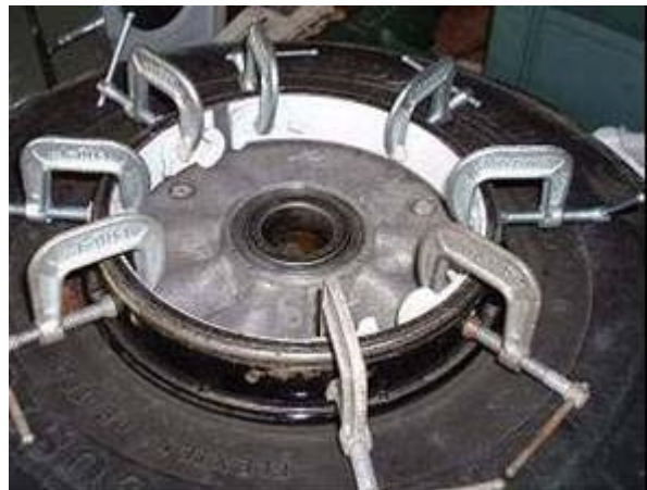
Figure 14 Clamping new lining using brake shoes.
