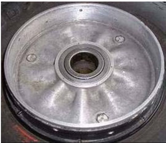
Figure 13 Cleaned-up lining housing
